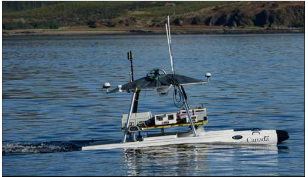
Defence Research and Development Canada's unmanned surface vehicle USV-2600 performs an autonomous mission in the water at Loch Alsh. – Photo by Janice Lang, DRDC
